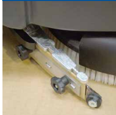
Tool less maintenance swinging squee-gee
